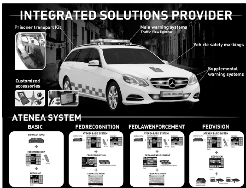
Pictogram showing the functioning of the ATHENA system.
